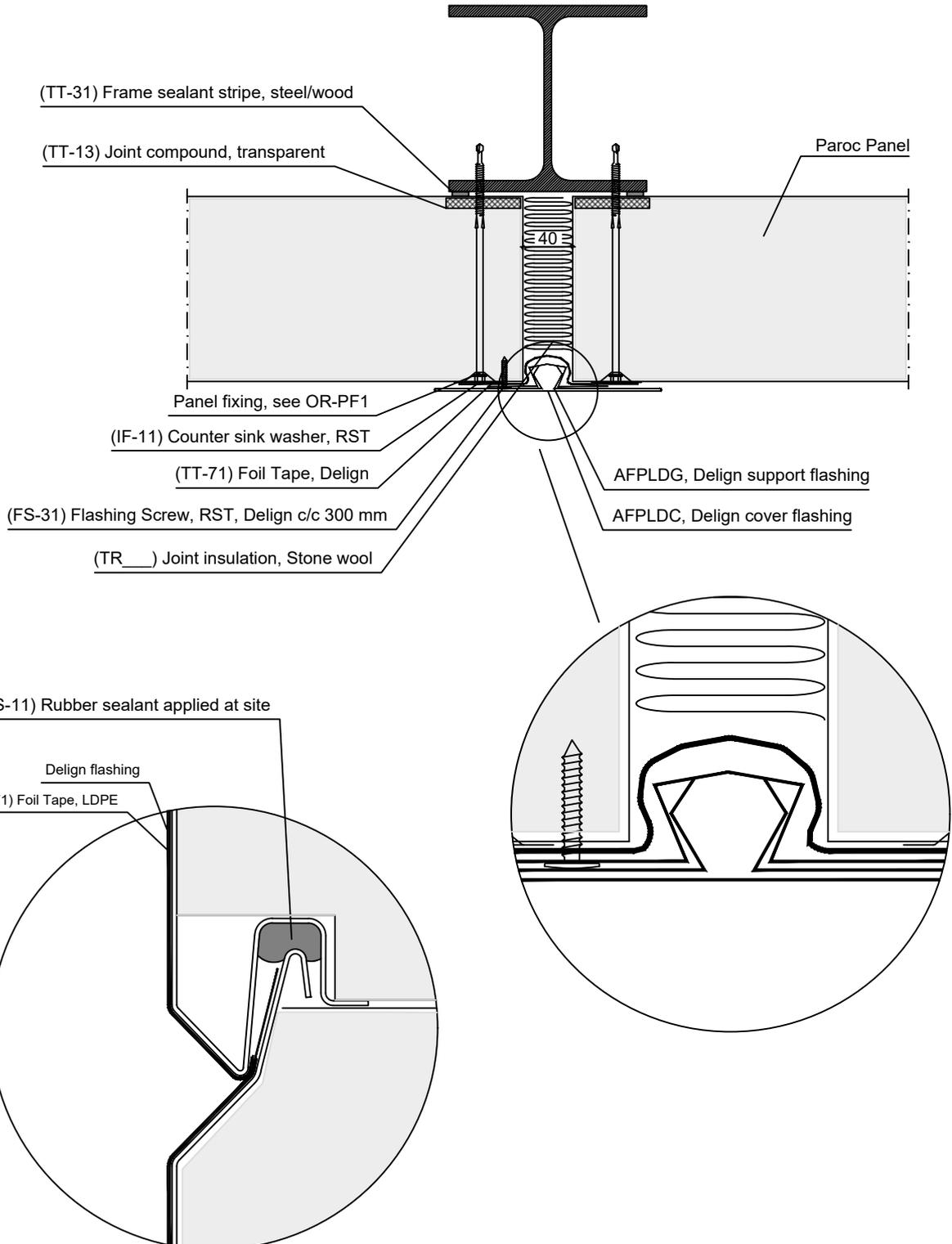
This detail has been done to help architects, engineers and installers when using PAROC panels. Before using this detail, check latest version at [www.parocpanels.com](http://www.parocpanels.com)
