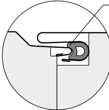
Factory applied sealant or joint compound (TT-13)
