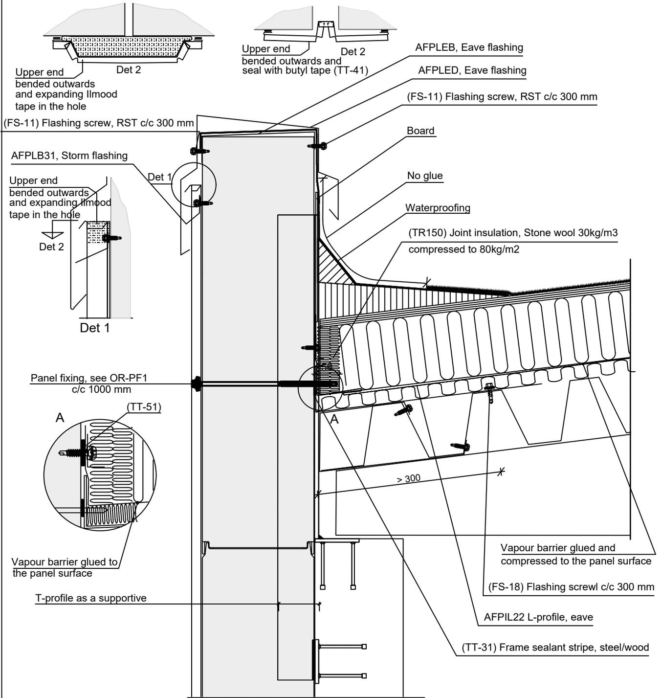
If concrete columns cast without welding plates, use chemical anchor to fasten the T-profile.
