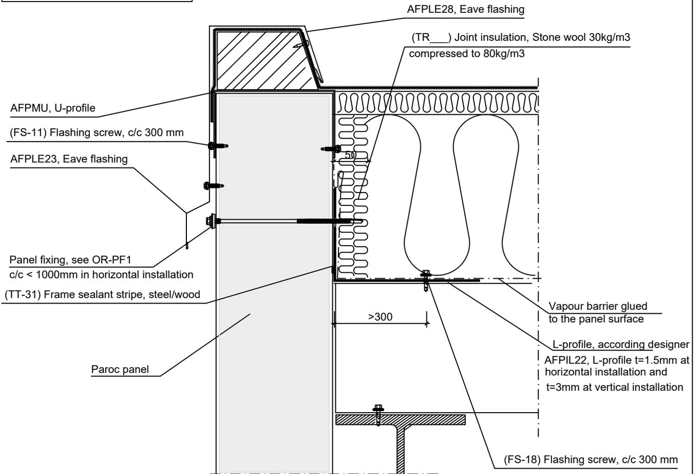
This detail has been done to help architects, engineers and installers when using PAROC panels. Before using this detail, check latest version at [www.parocpanels.com](http://www.parocpanels.com)
