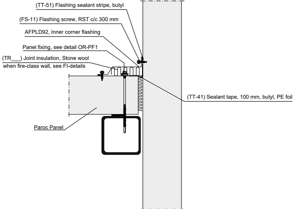
This detail has been done to help architects, engineers and installers when using PAROC panels. Before using this detail check latest version at [www.parocpanelsystem.com](http://www.parocpanelsystem.com)
