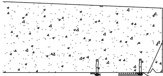
(FC-11) Spike, carbon steel, concrete c/c 400 mm
