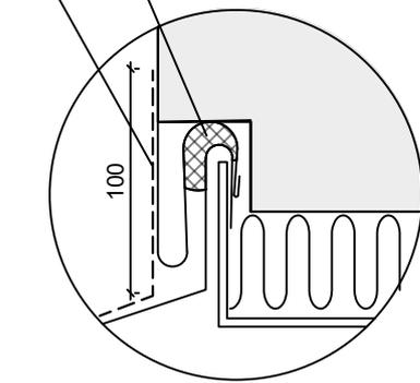
(TT-13) Joint compound, transparent or factory applied sealant
