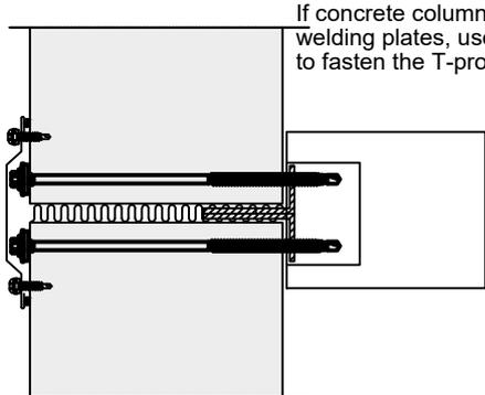
If concrete columns cast without welding plates, use chemical anchor to fasten the T-profile.
