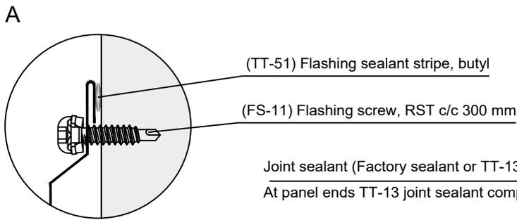
Joint sealant (Factory sealant or TT-13)
