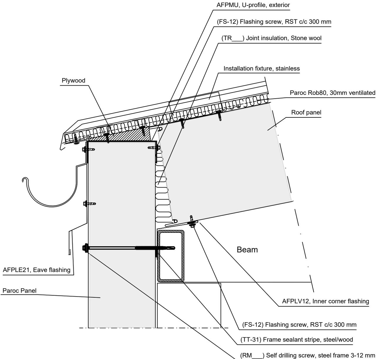
This detail has been done to help architects, engineers and installers when using PAROC panels. Before using this detail, check latest version at [www.parocpanels.com](http://www.parocpanels.com)
