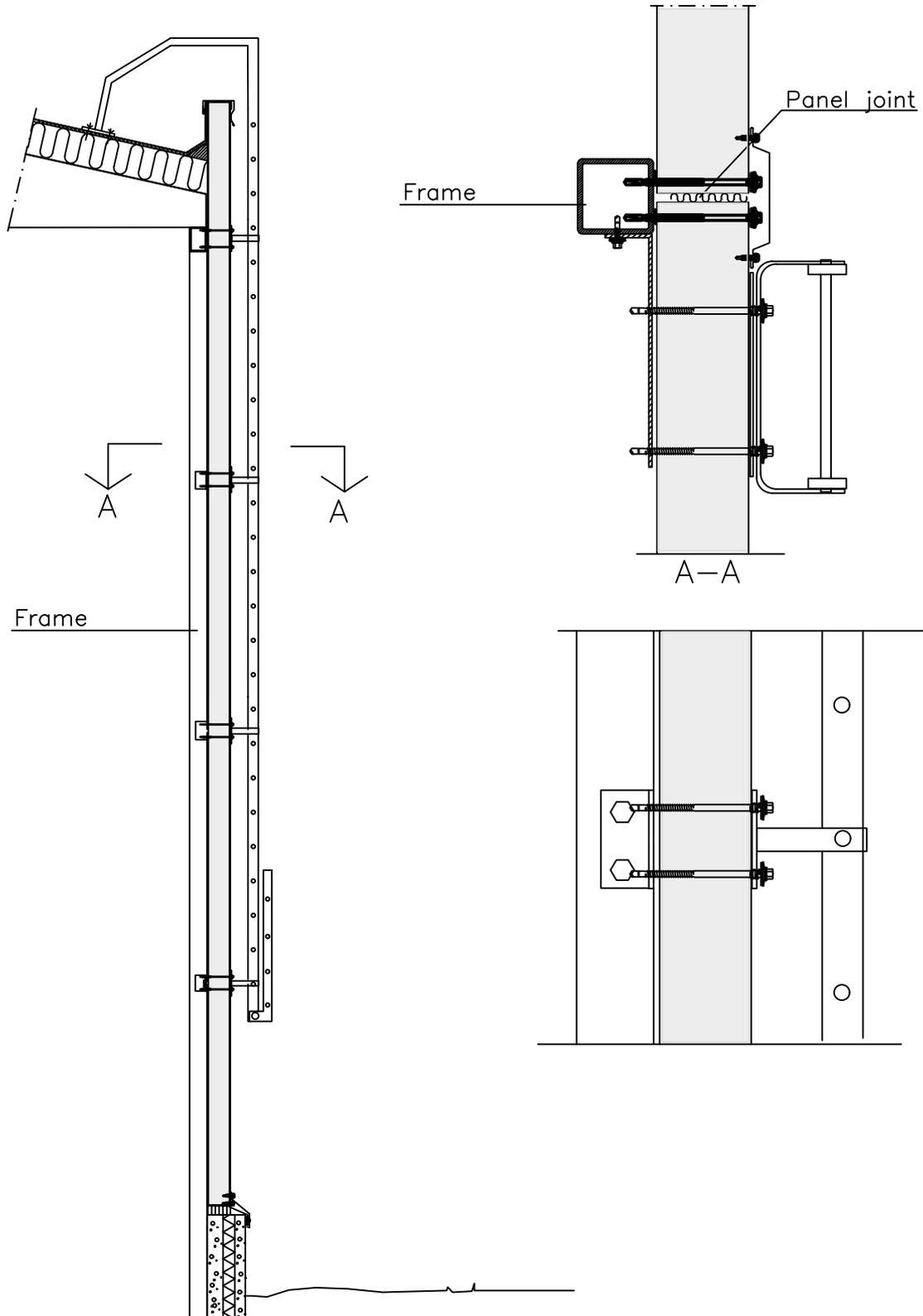
Upper end of a ladder must be fixed to the roof construction.
