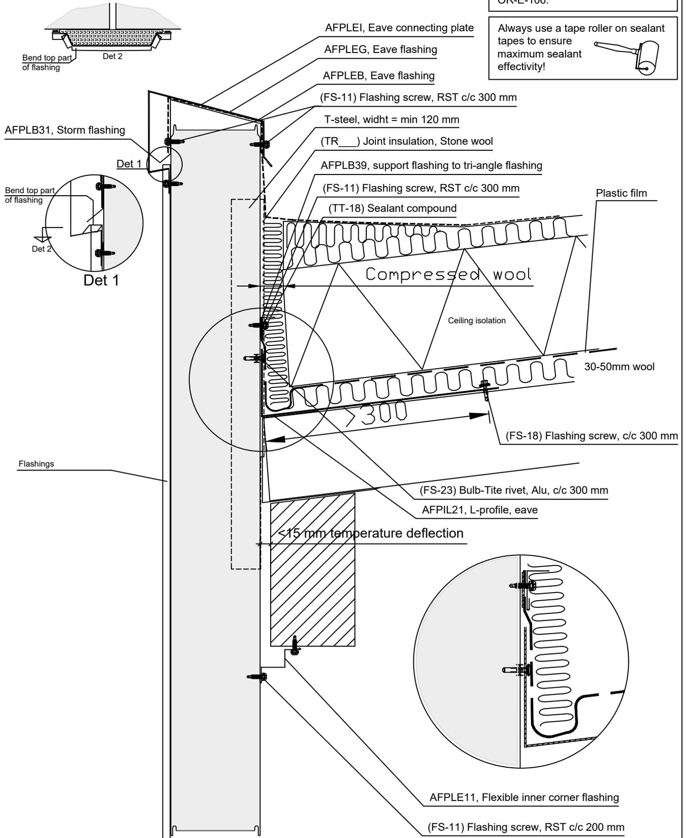
This detail has been done to help architects, engineers and installers when using PAROC panels. Before using this detail, check latest version at [www.parocpanels.com](http://www.parocpanels.com)
