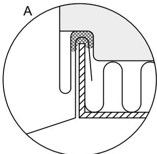
This detail has been done to help architects, engineers and installers when using PAROC panels. Before using this detail, check latest version at www.parocpanels.com
